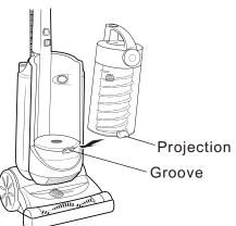
**2** Push the dust compartment into the main body as shown to reattach.
